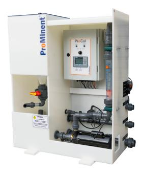
The ProMinent \* ProCal Granular Calcium Hypochlorite feeder generates a dilute solution from granulated dry chemical.
