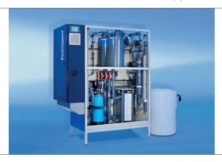
The CHLORINSITU® III range of electrolysis systems generates sodium hypochlorite with a concentration of 20-25 g/l without any significant leakage of sodium chloride from the electrolysis cell into the finished product. The pH value of the water being treated is affected substantially less than when conventional sodium hypochlorite is used (pH 12-13.5) owing to the moderate pH value (approx. 9). The result is a significantly lower quantity of chemicals needed to adjust the water's pH value.
