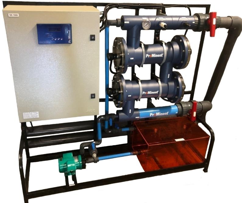
The ProMinent CSM-SS Salt Water Chlorinators feature a modular electrode design that incorporates the latest information technology through a digital LCD interface screen with user friendly menus, alarms, data logging, water flow and temperature monitoring, power supply temperature monitoring and the ability to control the output by an external water chemistry controller.
